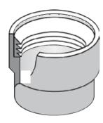
4. Depress the seal to ensure that it is correctly seated against the ledge of the fitting.
