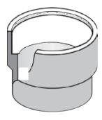
Examine the ledge inside the fitting to ensure that is free of dirt and debris.
