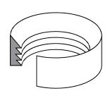
Obtain the TriSeal® and check that it is in the correct configuration with the ribs pointing inside. (If the TriSeal® is not in the correct orientation, twist it inside out to correct it.)
