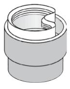
Deform the TriSeal® into a kidney shape and place it (flat end first) into the fitting. When in position, snap the seal in place against the fitting along its entire circumference.
